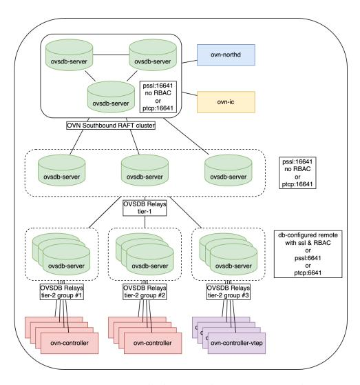
This deployment scenario can be useful if the count of OVSDB Relay groups from previous (multi-group) scenario becomes an issue for the OVSDB cluster and brings unwanted load on it. Deploy an intermediate group of OVSDB Relay servers to have just N connections on the cluster ovsdb-servers (where N is a number of Relay servers in this group), while other OVSDB Relay groups connect to this "intermediate" group.
