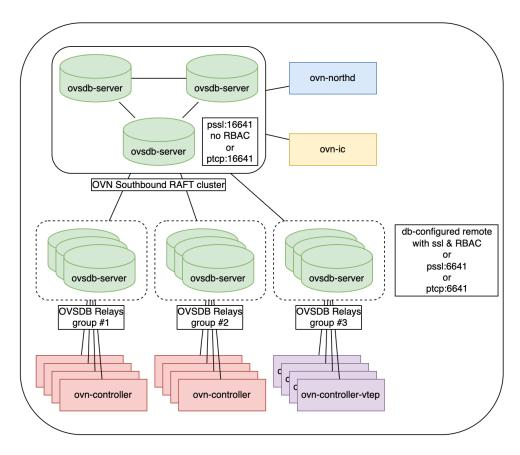
The difference between this deployment option and "one-group" is that it is possible to dedicate different groups of OVSDB Relays to serve different sets of ovn-controllers.
