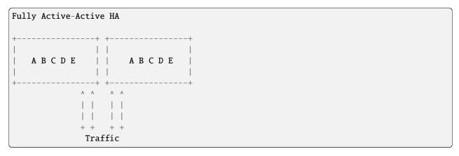
The final step in L3HA is to have true active-active HA. In this scenario each router has an instance on each Gateway, and a mechanism similar to ECMP is used to distribute traffic evenly among all instances. This mechanism would require Gateways to participate in routing protocols with the physical network to attract traffic and alert of failures. It is out of scope of this document, but may eventually be necessary.
